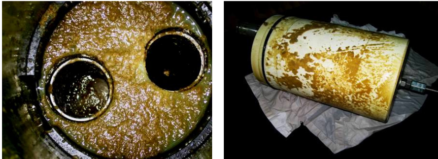
Figure 4.25: The pressure exchanger internals contaminated with slimy biofilms
