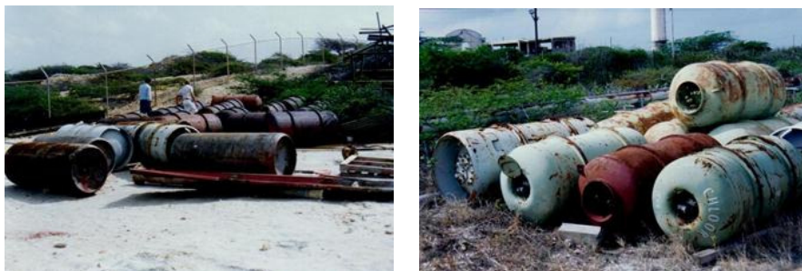
Figure 9.1: One-ton chlorine containers stored on the premises of W.E.B. Aruba N.V.
