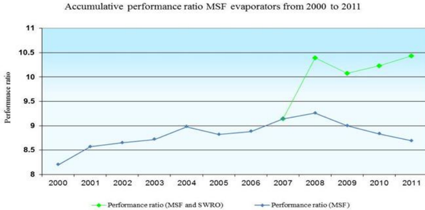
Figure 3.12: The trend of the performance ratio of the desalination units from 2000 to 2011
