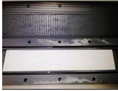
Membrane Fouling System
