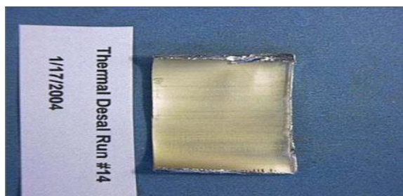
Figure 5.22: Deposits formed with 8 ppm active blend containing the new polymeric Phosphonate [5.6]
