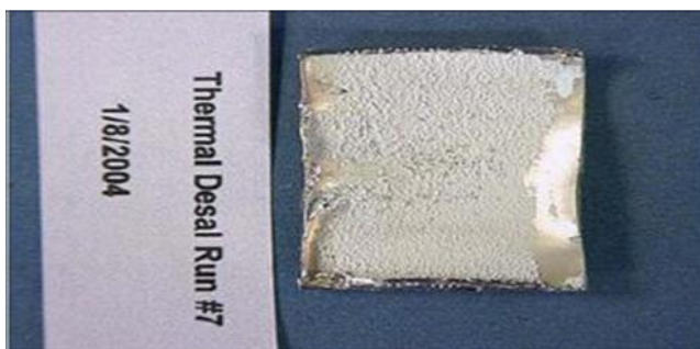
Figure 5.20: Heavy deposits on the test tube of the heat transfer surfaces during the control test [5.6]
