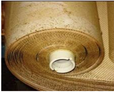
Disassembled biofouled membrane
