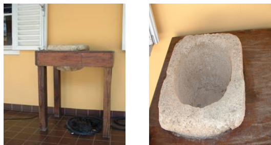
Figure 2.22: The Cudi used for filtering out suspended particles
